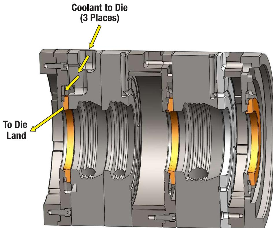
The teeth in the Lube Ring control the distribution of coolant to cover all working surfaces of the ironing die.
