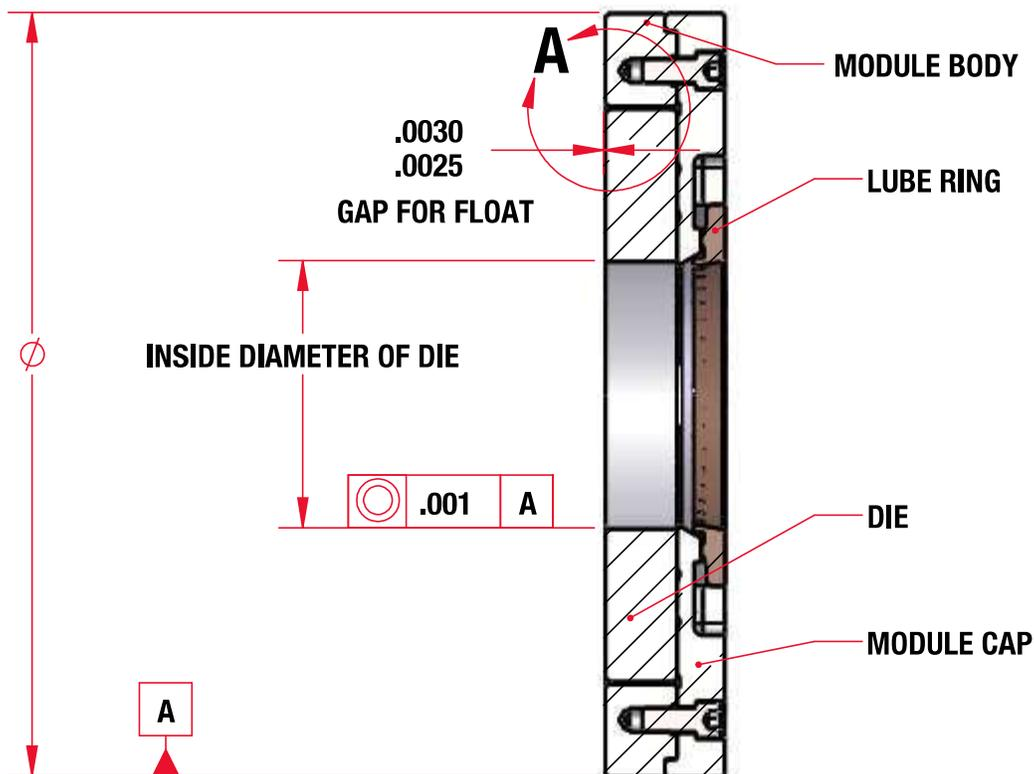
If the new pins and springs do not return the Module to center you will need to look at the Module. The Module rests on the bodymaker's two cradle rails. After prolonged use, the Module will wear where it rests on the cradle rails.
