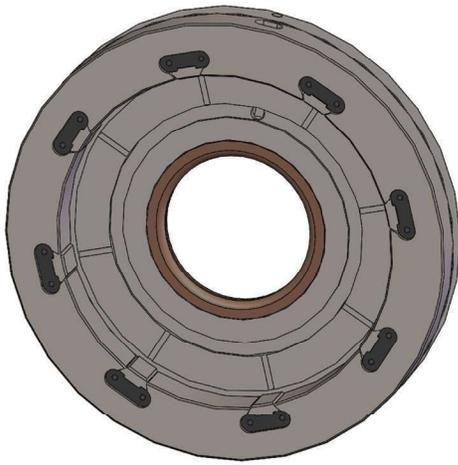
See air grooves in Module to break the vacuum behind the die.
