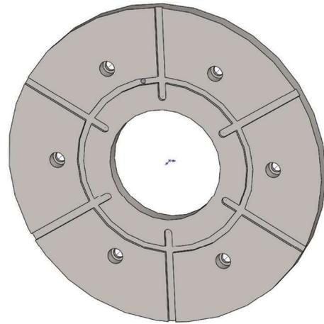
When the last die in the Tool Pack rests against the bolster plate, the vacuum must be broken by charging the grooves with air pressure in a plate added to the bolster.
