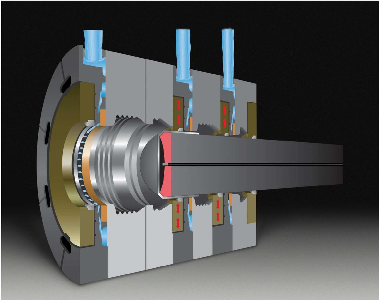
The Pride Floating Tool Pack uses a die suspension system with springs and pins mounted in a precision Module to support the ironing die. The Pride floating suspension system allows the ironing die to move to align with the punch instead of forcing the punch to align with a fixed die. Pride's system of floating the ironing dies reduces stress on both the can wall and tooling.
