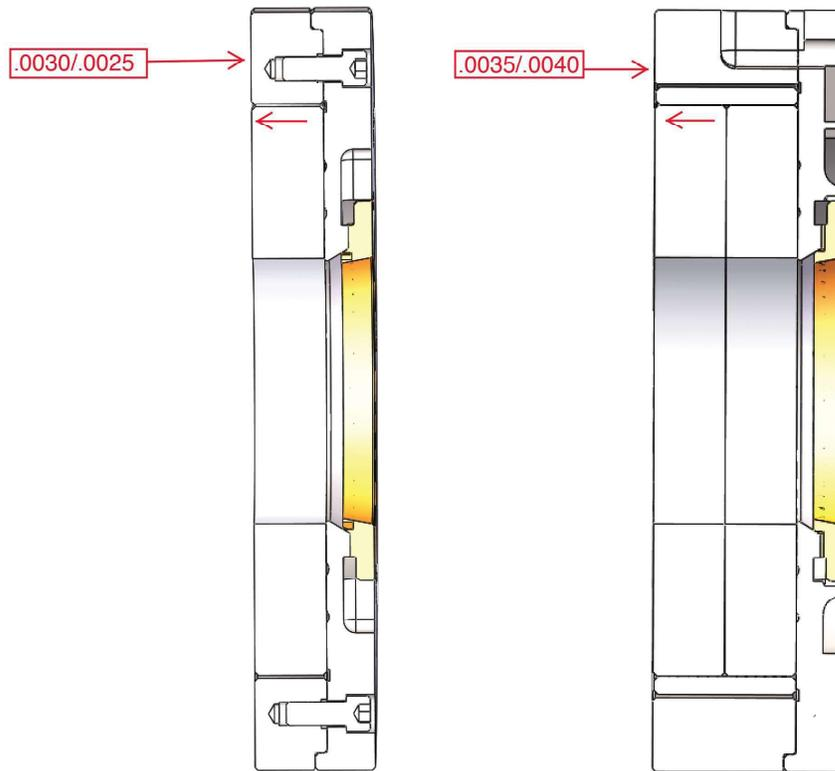
Check the flatness of surfaces that contact the die including the inside of the Module and adjoining spacer surfaces. The die should sit in a single die Module at a minimum of 0.0025" (0.063mm) below the surface and a minimum of 0.0035" (0.089mm) of a double die Module.
