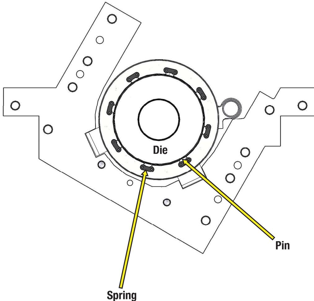
The springs and pins can easily be removed with a small flat head screwdriver. Carefully pry the pin out by inserting the flat head screwdriver under the pin and lift it out of its machined pocket. Once the pin is removed, push a small screw driver into one of the two holes of rubber spring and lift it out. Take care not to scratch or nick the Module with the screw driver.
