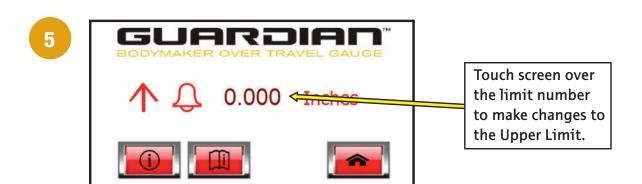
**UPPER LIMIT:** Most can makers set the upper limit parameter so that a double can will trigger the Portable Guardian to issue an upper limit error alarm.
