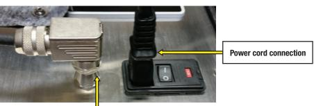
Connect sensor to Portable Guardian by inserting the sensor connector into its mating half in the Portable Guardian and hand tightening the connector nut ring $^*$
