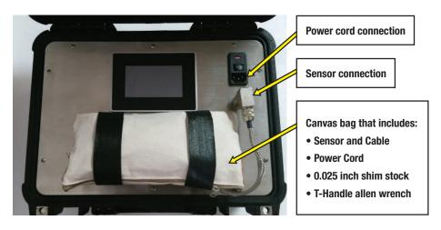
Connect the power cord and sensor to Portable Guardian
